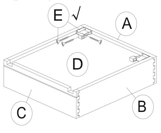
WARNING: FORBID SCREWING ON BOTTOM PANEL
