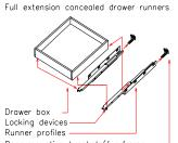
Runner profiles Rear mounting brackets(for frame applications)
